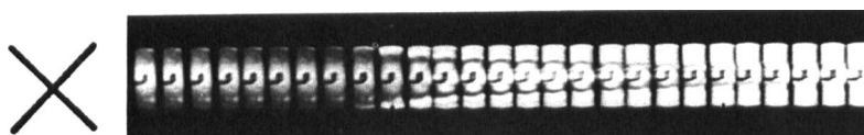
Figure 3. Interference patterns in stage I of the intermediate and high p regimes ( p > p_1 ). p = 3.0 cm Hg, \Delta t = 0.0155 s.
